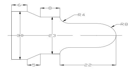
2. Using Stock removal cycle – Create a part program for multiple turning operations and produce component in the Machine.
