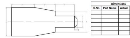
2. Prepare the specimen and make the Step Turing & Thread cutting as shown in figure using the Lathe.
